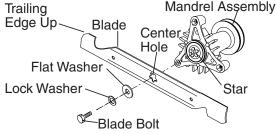
If bolt needs replacing, replace only with approve bolt shown in the Repair Parts.
